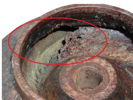
Figure: Impeller damaged by cavitation
