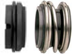
Rubber bellow seal: For liquids with fine solids, for general applications like water pumping solids
